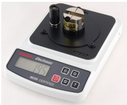
Figure 17: Visual of testing apparatus. After zeroing device, insert edge onto chrome colored portion and record result.
